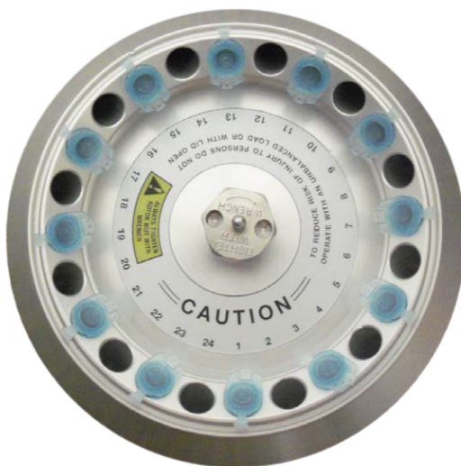
Figure 1. Loading the rotor to achieve balance.
